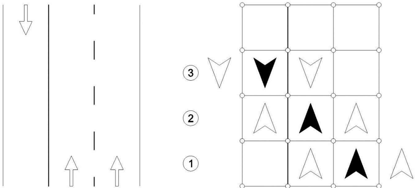
**Fig. 2.** Scheme and usage of the newly developed map model. Situation with the lane markings and the driving directions (left figure) and the corresponding topology with the mesh cells (right figure). Black arrows are for the analysed vehicles, white arrows for the possible lane changes. Numbers represent the scenarios
