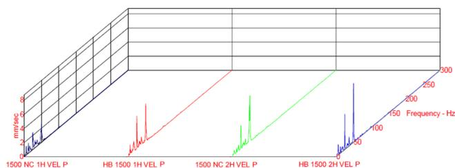
Fig. 7. Effect of exhaust clogging on vibration spectrum
