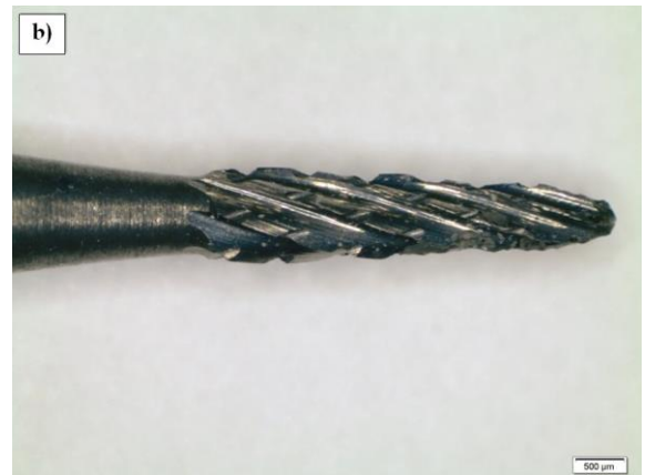
Fig. 1. Tungsten carbide dental bur after use: a) all shape, b) bur head (the cutting edge)
