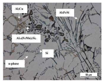
Fig. 1. Microstructure of AlSi6Cu4 alloy (alloyed by master alloy AlFe10) without vanadium, etch. H<sub>2</sub>SO<sub>4</sub>
