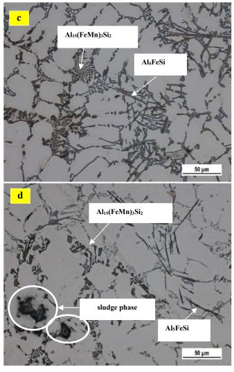
**Fig. 2.** Effect of V to morphology of Fe-phases, etch. H<sub>2</sub>SO<sub>4</sub> a) 0.5% V b) 1% V c) 1.5% V d) 2 hm.% V
